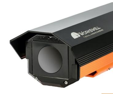
Workswell SAFETIS Outdoor camera offers great resolution of 640 x 512 px, sensitivity of 50 mK (0.05 °C) and fast response within milliseconds. The powerful communication interface allows connecting SAFETIS camera directly to any computer via Web-server or directly to SAFETIS Control Unit via Ethernet RJ45. The SAFETIS camera has integrated 7 digital outputs in the camera and 7 digital outputs in SAFETIS Control Unit that can be triggered at the same time if needed.
